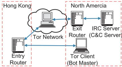
Fig. 17. Experiment setup for traceback.
