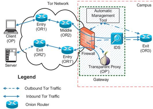
Fig. 3. System architecture for malicious traffic collection.
