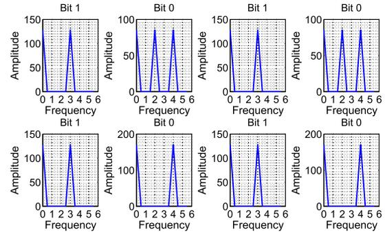
Fig. 18. Upper row: bits 1010 by feature frequencies 3 and 2 Hz; Bottom row: bits 1010 by feature frequencies 3 and 4 Hz.
