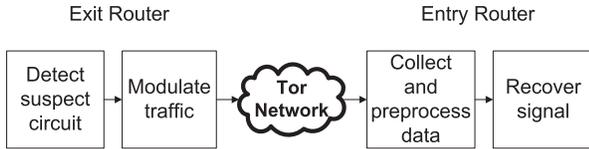
Fig. 13. Workflow of the DTMF signaling based approach.
